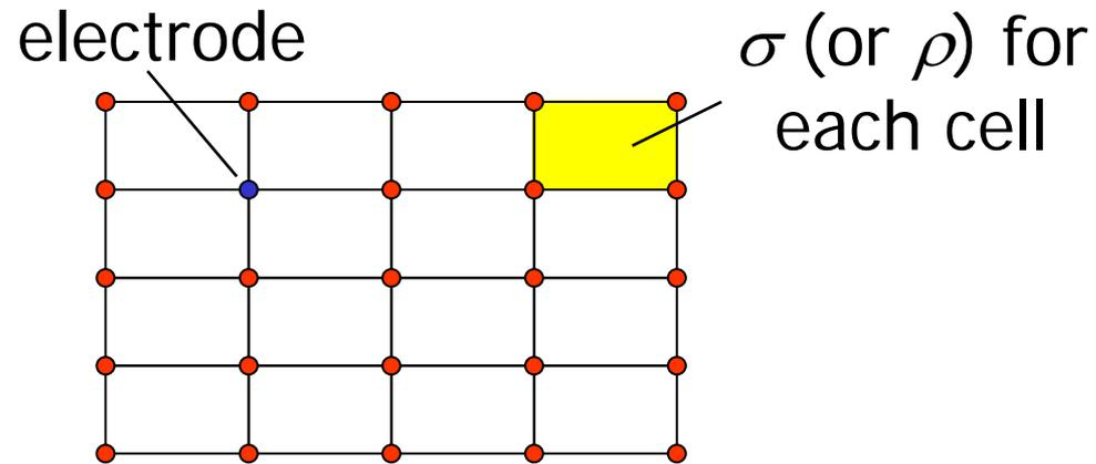
The forward equations are solved for current injection at each electrode.
