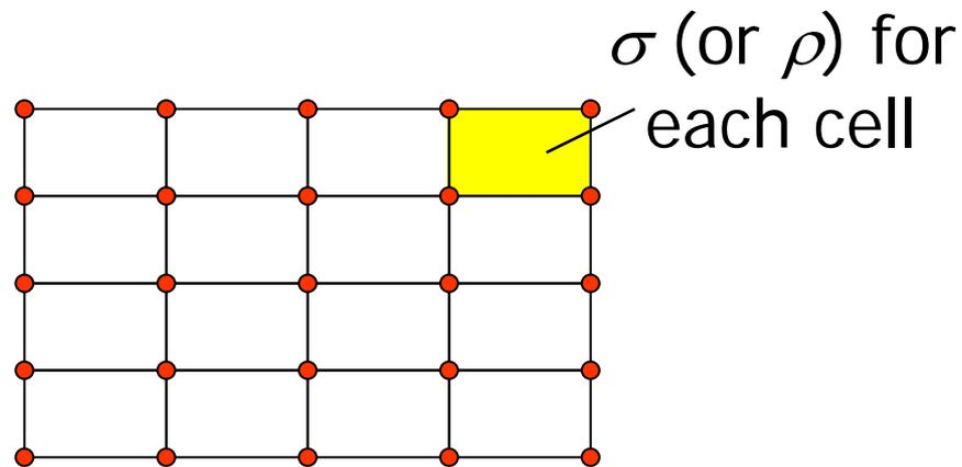
Electrode are located at node points and hence potentials may be determined at electrodes.
